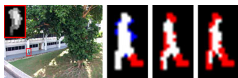
Fig. 6. Combining one-pass RPCA with motion saliency filtering. From left to right: saliency of the human figure with brighter intensity denoting higher saliency values; results of foreground detection, with \lambda = 0.5, 1 , and 2 respectively.
